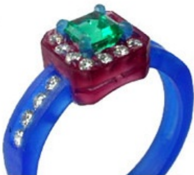
In stone-in-place casting, gems are first set in a wax model of the piece to be cast. Photo by Dr. Hubert Schuster, courtesy Neutec.
