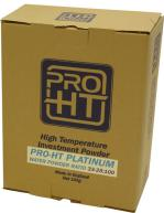
Pro-HT is a high technology phosphate bonded product designed for casting high temperature alloys such as Platinum and Steel with metal pouring temperatures up to 2100°C / 3800°F. Pro-HT has a high refractory content and fine particle size distribution, this produces high fired mould strength with precise detail replication of the wax pattern under the harsh casting conditions these alloys demand.
